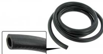
Brandstofslang textiel versterkt per meter Binnendiameter: 8.00 (max. 8.50mm), Buitendiameter: 13.70 (max. 14.20mm), Working pressure: 7.5 bar, Bursting pressure: 30 bar
